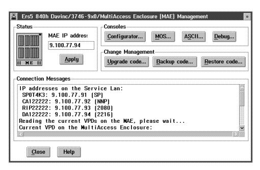
\_\_ 2. When requested "Insert" the new MAE optical disk (PN 08J5473). Then, click on OK.
